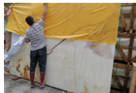
1. Covering the slabs by masking tap
