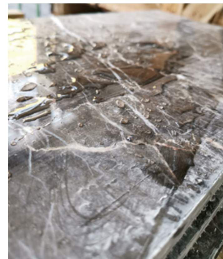
3. Water proof testing
